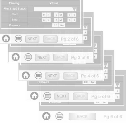
Once programming is complete, the 1<sup>st</sup> page of the timing group shows how many Stages are active AND which Mode they are set to.
