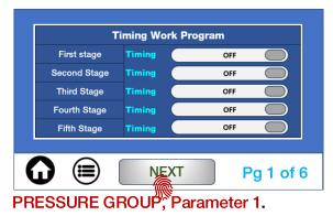
**Timing Work:** the controller will ONLY operate at the times and pressure(s) set at each stage
